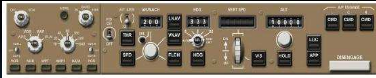
Master Control Panel
